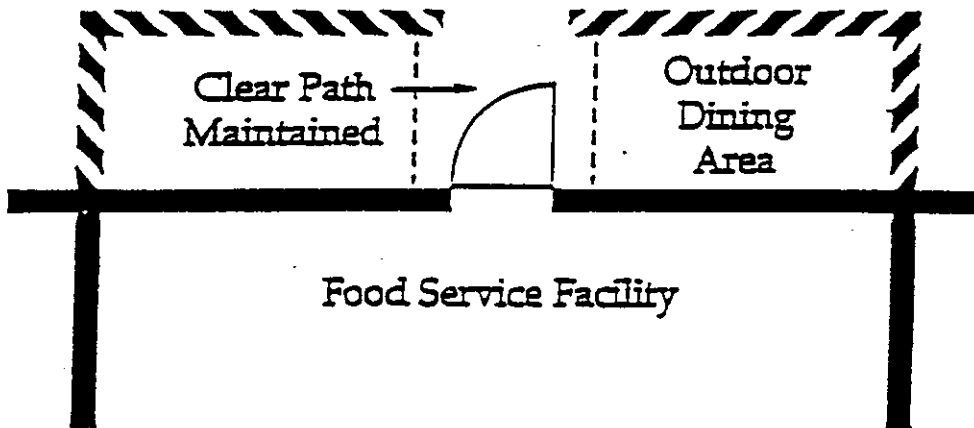
Clear Path To Entry Shall Be Maintained
